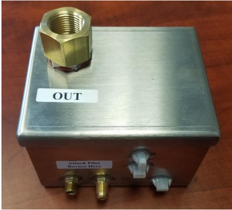
Ignition Control Box with Brass Extension
