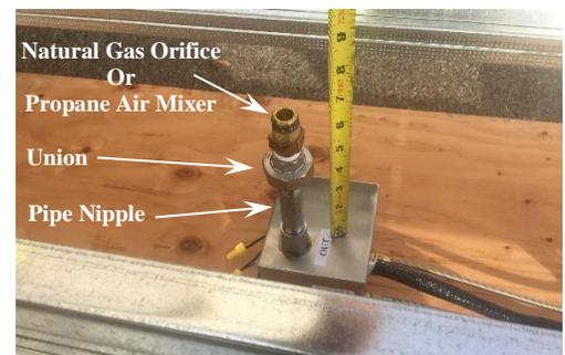
9. Remove the top half of the Union along with the orifice threaded into it. Apply Teflon Tape or Pipe Dope (suitable for Natural Gas or Propane applications) to the orifice and thread it into the Gas Inlet of the Burner.
