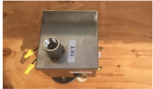
6. Attach the Pilot Burner. On the side of the Ignition Control Box there are two brass fittings and a white electrical connector for the Pilot Burner.
