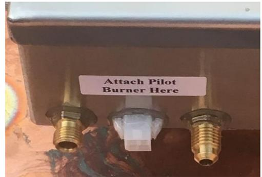
7. After connecting the Pilot Burner to the Ignition Control Box bend the gas lines such that the Pilot Burner is up near where it will end up when the Burner Pan is installed. When you are done manipulating the Pilot Burner it should look similar to the photo at right.
