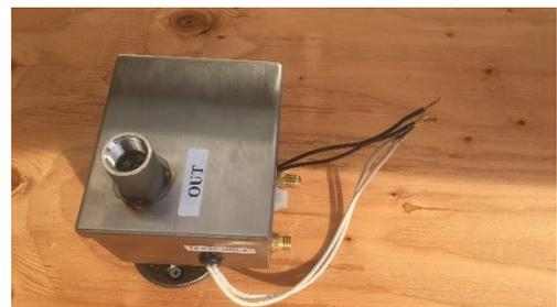
5. Using wire nuts attach the wires from the Ignition Control Box to the 12-gauge wires installed in the fire feature. We recommend partially wrapping the wires around the gas riser underneath the Ignition Control Box as shown. This will protect the electrical connections from the radiant heat from the feature.
